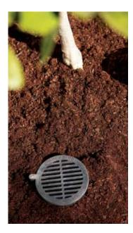
The Root Watering Series (RWS) product consists of a perforated polyethylene cylinder with an integrated bubbler and optional check valve. It is an excellent point source irrigation device for both trees and shrubs. It easily connects to turf irrigation lateral lines; or can be installed with drip zones. The RWS promotes deep root growth and healthy tree development and is appropriate for installation in both residential and commercial irrigation systems.
